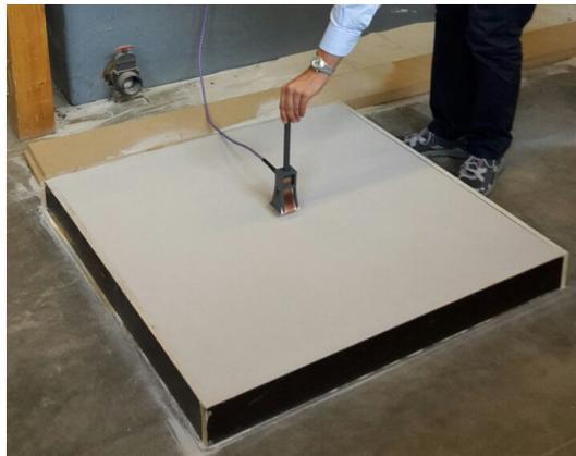
**FIG. 2** – Measurements in small sand box with different volumetric water contents.
