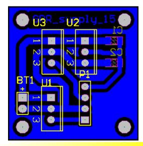
Warning! We recommend not welding directly to the copper layer the TSRN 1-2465 converters that do not tolerate high temperature.
