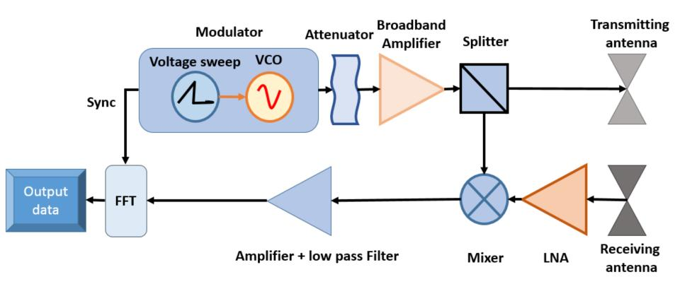
FFT and Output data blocks are carried out inside the PC
