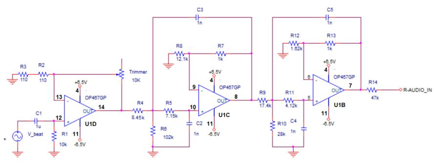
The amplification is set by the trimmer and the filtering modules determine the maximum bandwidth frequency around 15 kHz..
