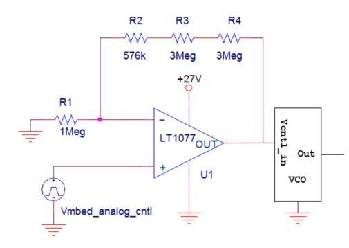
Values of the resistors result in an amplification of the noninverting stage equal to Av = 7.576
