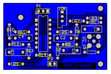
Connect «+ out» pin of connector P2 by means of a wire to the right channel of the laptop audio input. The same connector jack used for the mbed board («+ Sync pulse» signal).
