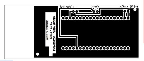
COST is supported by the EU Framework Programme Horizon2020 Vcc should be selected in the range 4.5V÷9 V. You can select one of the two +5V or +6.5 V voltages generated by DC-DC converter (circuit No. 1).
