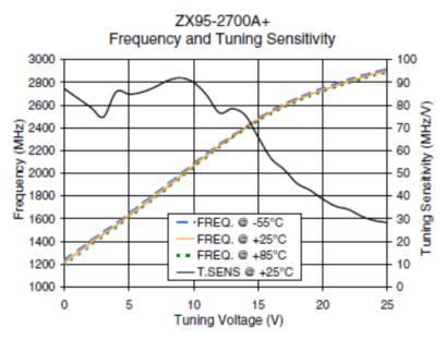
In the case of triangular FM, the nonlinear characteristic <<tuning voltage-frequency>> of the VCO imposes the use of a control voltage waveform different that triangular for compensating the compression showing at higher voltage values.
