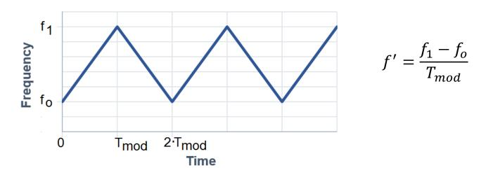
Transmitted signal is a frequency modulated sine wave
