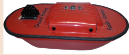
Antenna: Radarteam SUB-ECHO HBD 300 Central frequency: 300 MHz 3-dB BW: 120-780 MHz 4 kg, 72x36x16 cm
