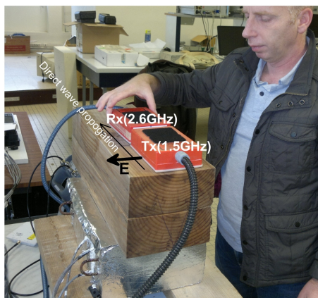
Direct wave, E vector perpendicular to fibers Distance TxRx, 16-26cm
