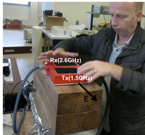
Direct wave, E vector parallel to fibers Distance TxRx, 11-21cm
