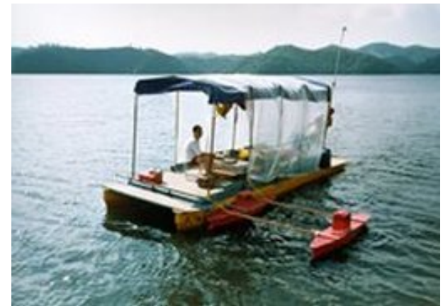
GPR prospecting on a lake (image courtesy of GeoScan Subsurface Surveys)
