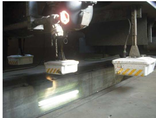
Fig. 8. GPR antennas: air-coupled (right) and ground-coupled (left) configurations.
