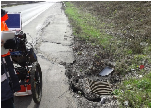
Hole detection on BRRC test track ("deep" hole, air void)
