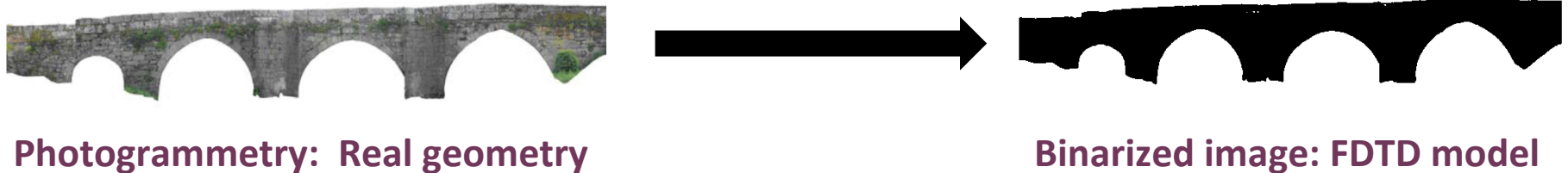
Fig. 9. Binarized image used as input to create the synthetic model.
