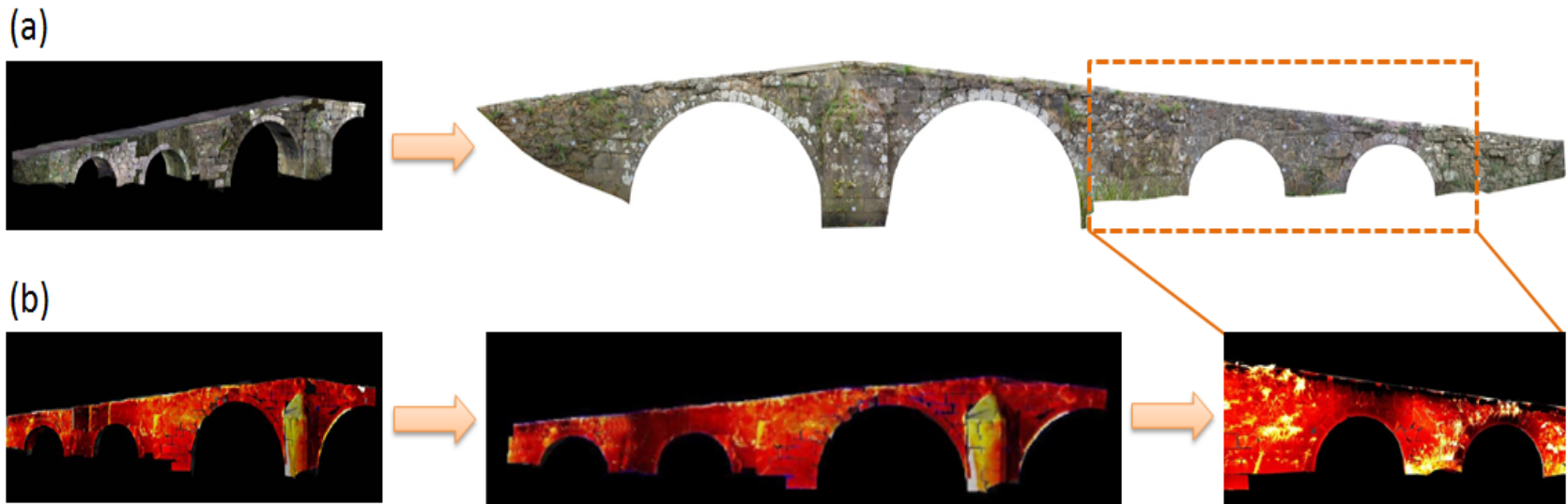
Fig. 15. Results of the geomatic surveys: 3D model with RGB (a) and thermographic (b) texture (downstream view).
